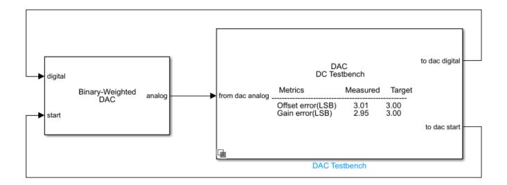
The measured offset and gain errors are displayed on the icon of the DAC Testbench.
