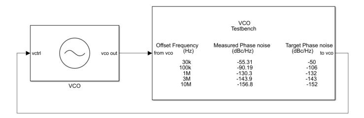
In the **Block Parameters** dialog box of VCO, click the **Plot measurement** button to plot the phase noise profile of the VCO. Notice that the VCO operating frequency is 3 GHz, and that the measured and targeted phase noise profiles match.
